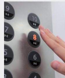
Business Management Department Touchless hybrid elevator switches used for an elevator at GINZA PLACE, an integrated commercial facility at the Ginza 4-chome intersection
