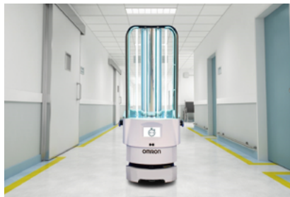
Mobile robot equipped with UV light irradiator to prevent infection
