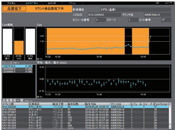
Fig. 12 Case of quality deterioration detection 2
