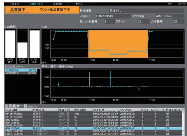
Fig. 11 Case of quality deterioration detection 1(2)
